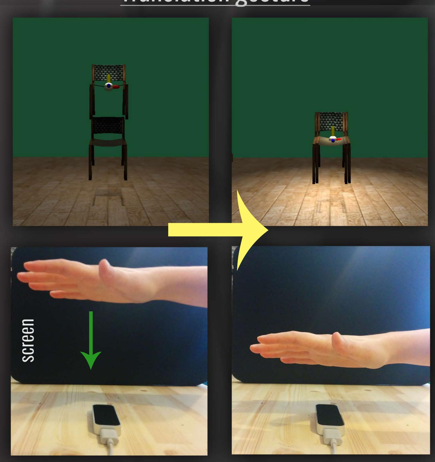
The hand has full control over the three axes (X Y Z) when translating
