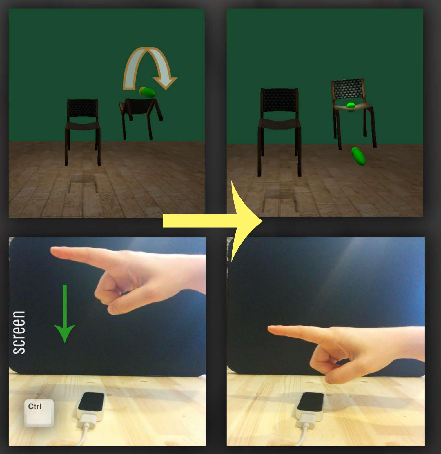
The finger's translation rotates the chair in an axis perpendicular to the direction of the movement of the finger
